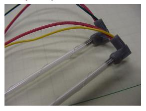
Figure 8. Lamps Wrapped with Instant Lamp Warmup Wiring
